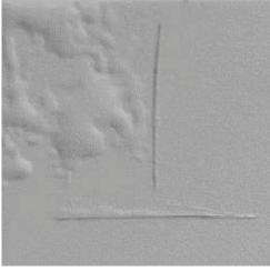
**EXAMPLE PASSED TEST** No bubbles, uneven surfaces or corrosion marks were found after 1500 hrs
